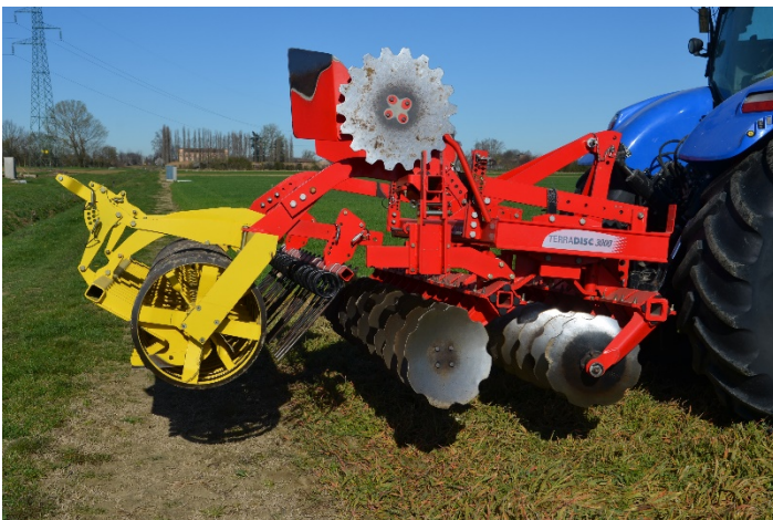
Figure 8 – Disc harrow to achieve minimal soil processing
